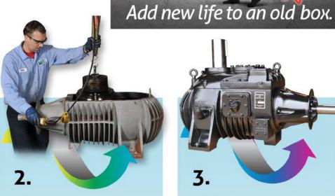
After receiving your drive, an Amarillo<sup>®</sup> Gear Technician will inspect for wear and damage. We will then send you an As Found Condition Report, photographs of critical wear parts and an exact cost for renewal of your gearbox.
